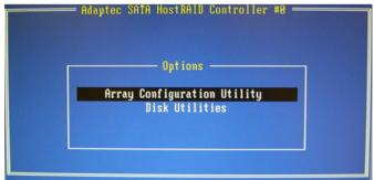
Press <Ctrl><A> for Adaptec RAID Configuration Utility
